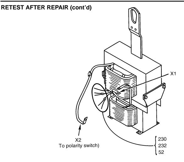
FIGURE F.16 - TRANSFORMER LEAD TEST POINTS.
